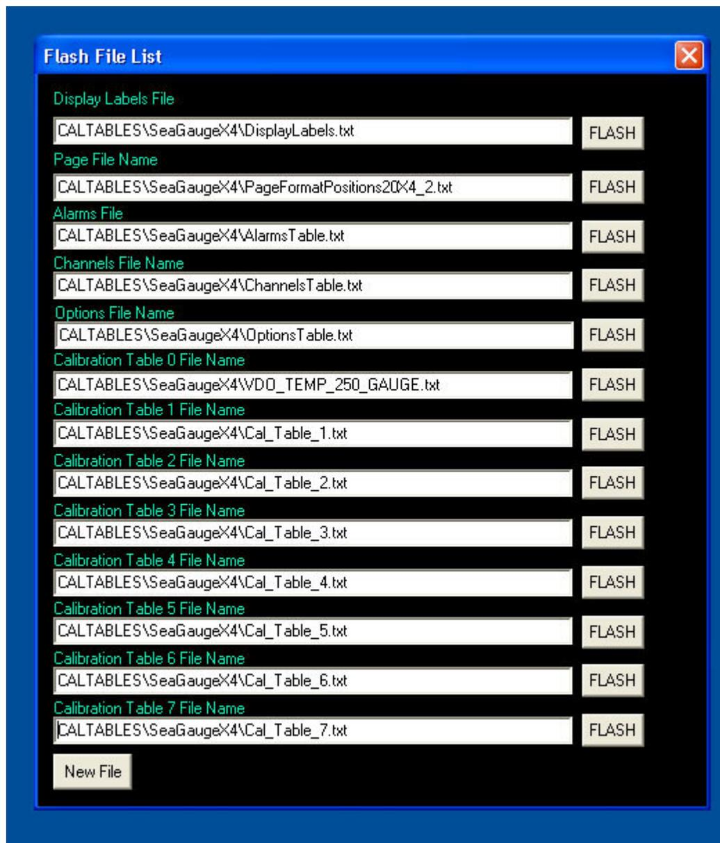
All configuration data is stored in text files for FLASH memory programming of attached vGauge units. To update unit, simple click the appropriate FLASH button.
