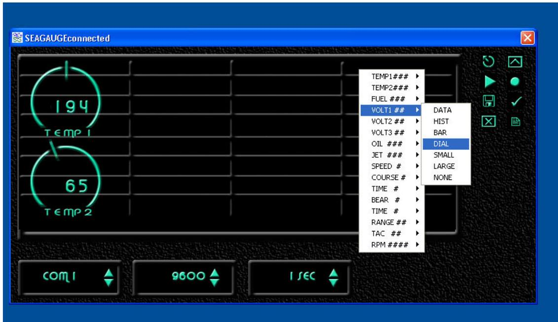
To place display graphic element on virtual dashboard page, simply right click mouse button and pick the sensor label and display mode. The selected item will appear at the grid point of the mouse position.
