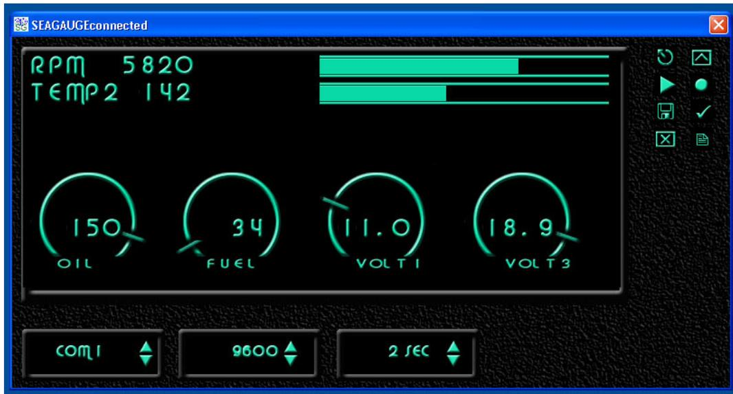
Graphic display modes can be mixed in any combination to create the desired display format.
