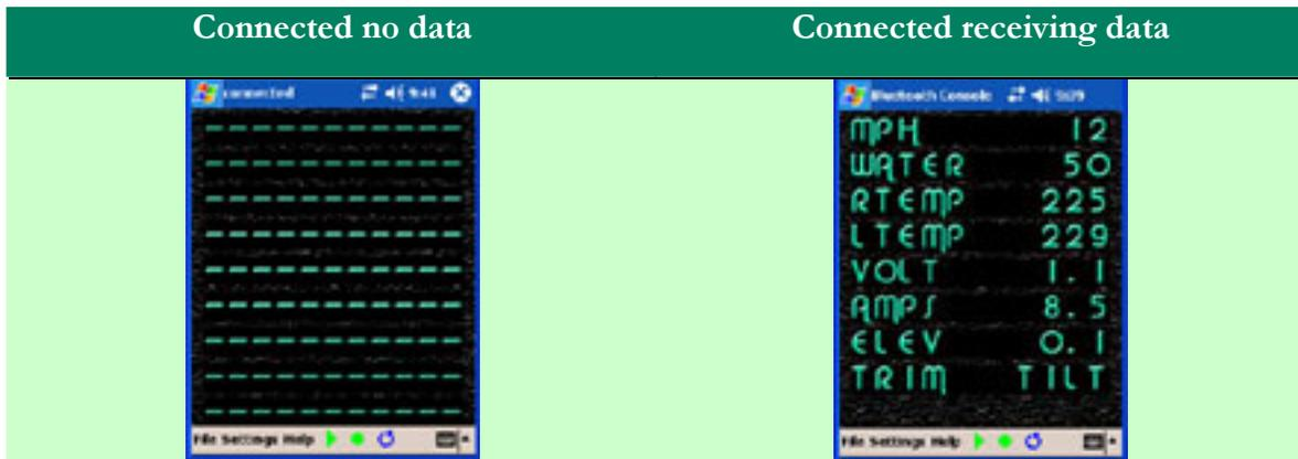
After successful connection the TITLE BAR will display “Connected”. When NMEA data starts arriving the TITLE BAR will display the name of the device sending data SeaView will decode compatible NMEA data and display the device labels on the left and sensor data on the right. SeaView will display the first 7 characters of device labels and the first 4 characters of sensor data.
