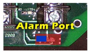
Open Collector Ground drive. Open circuit when alarm off, sink to ground when alarm on. Used to ground relay to drive higher current device. Sinks up to 100 mA
