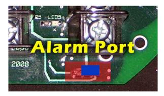
Voltage Drive mode. 0V when alarm off, 3.3 volts when alarm on – Drive small Pizo buzzer or reed relay. Source 50 mA
