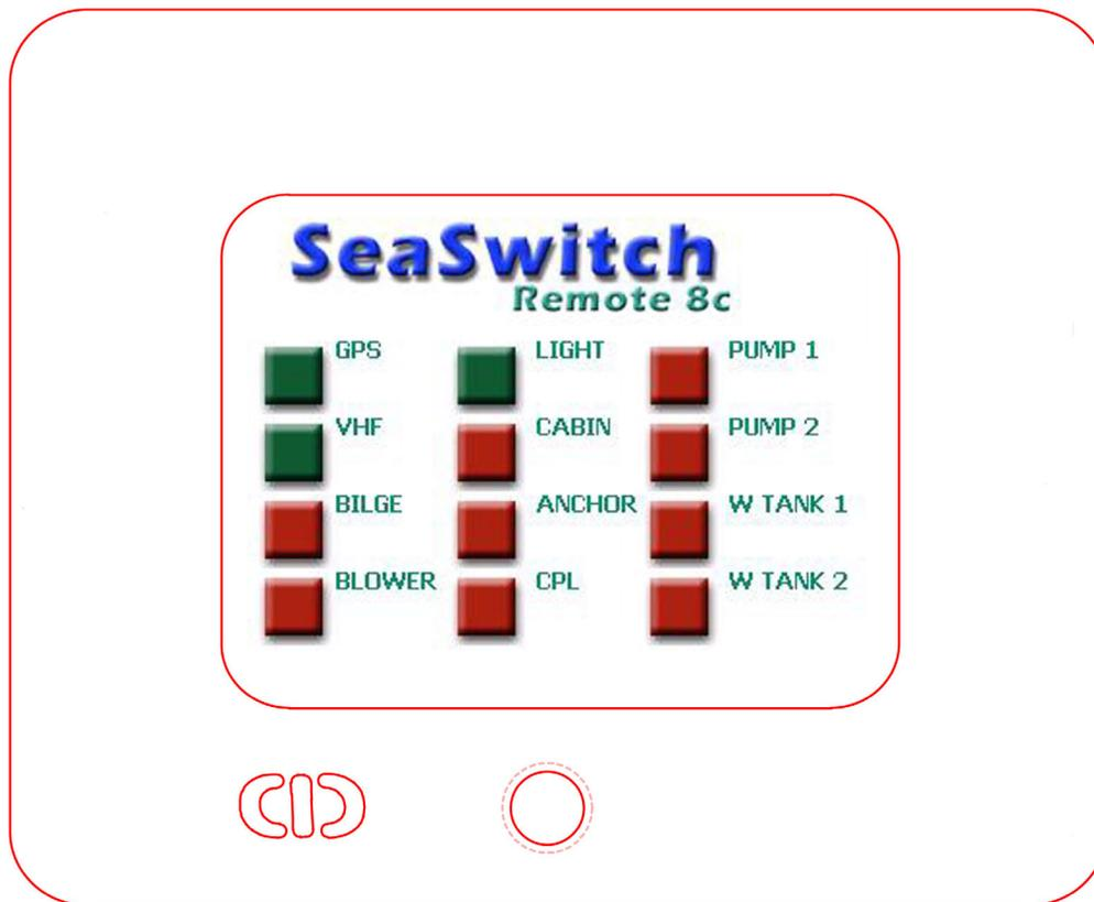
The Switch display names are programmed into the vGauge Remote Sensor unit during initial configuration. Switch names can not be directly altered by the G12C display head. Switch names can be easily modified using the vDash configuration utility.
