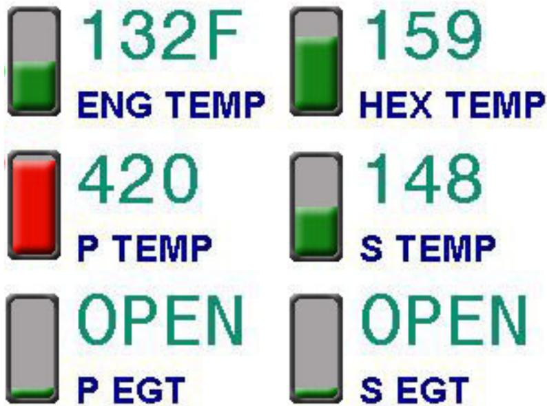
All graphic elements are pre-loaded in G12C Flash memory to speed display updates. Different display themes can be created by loading new graphic elements in G12C Flash memory using an Firmware Update utility without effecting any programming or configuration of vGauge Remote sensor unit.
