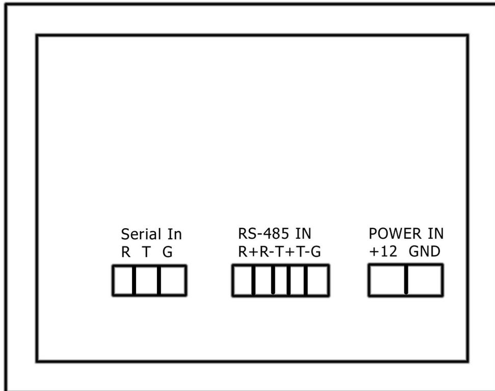
Power Input should be switched and fused to 4 Amps.
