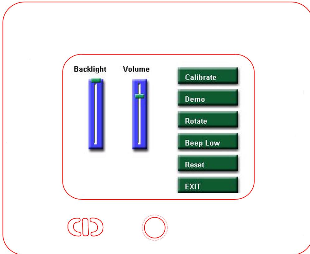
**BACKLIGHT ADJUST** – Touch Slider to allow adjustment of backlight brightness. Touch and drag down to dim or drag up to brighten.
