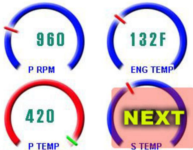
the G12C sends a command back to the vGauge Remote sensor unit to construct the next display page in sequence.
