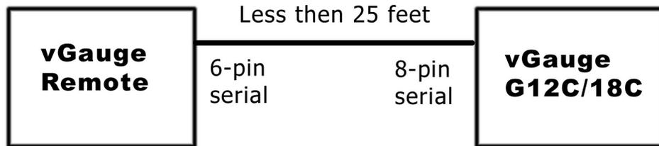
For distances longer than the specified 25 foot maximum, a separate power adapter will be required for G12C units. The adapter requires a switched 12 volt source located near the G12C display
