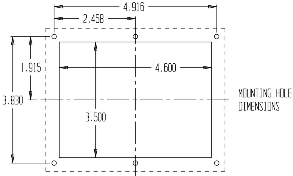
The unit can be secured in place by using bolts through the mounting holes. **Do not let the glass of the display touch the dash.** Use standoffs and foam tape to insulate the glass from the rear of the dash. The module should be suspended by the mounting bolts only.
