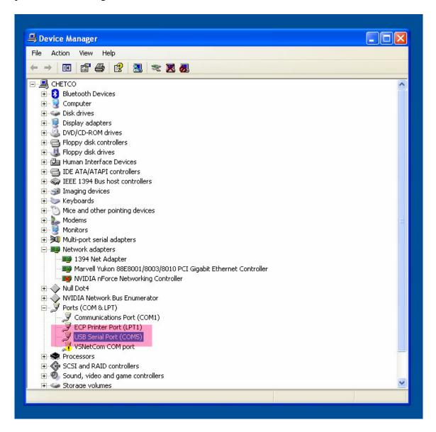
In this example - COM PORT 5 was assigned to the G24C display when the Serial to USB cable was attached to the host PC. Verify the correct COM port by disconnecting the USB cable and it should disappear from the list. Reconnect should reinstall the same COM PORT number.
