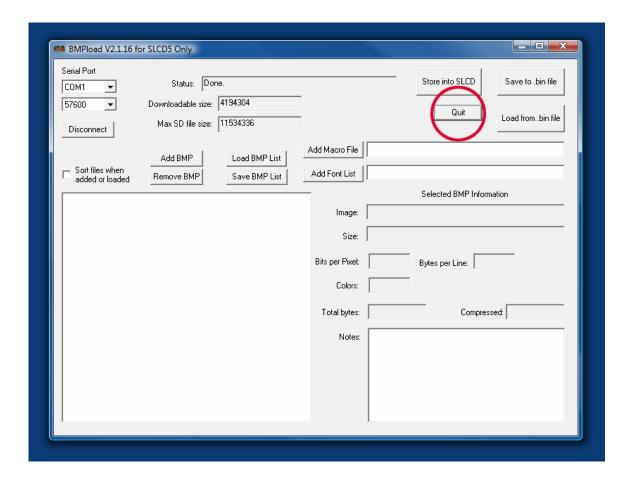
At this point you may disconnect the Serial to USB cable from the display and cycle power to reset and initialize at the new Baud Rate of 57600.
