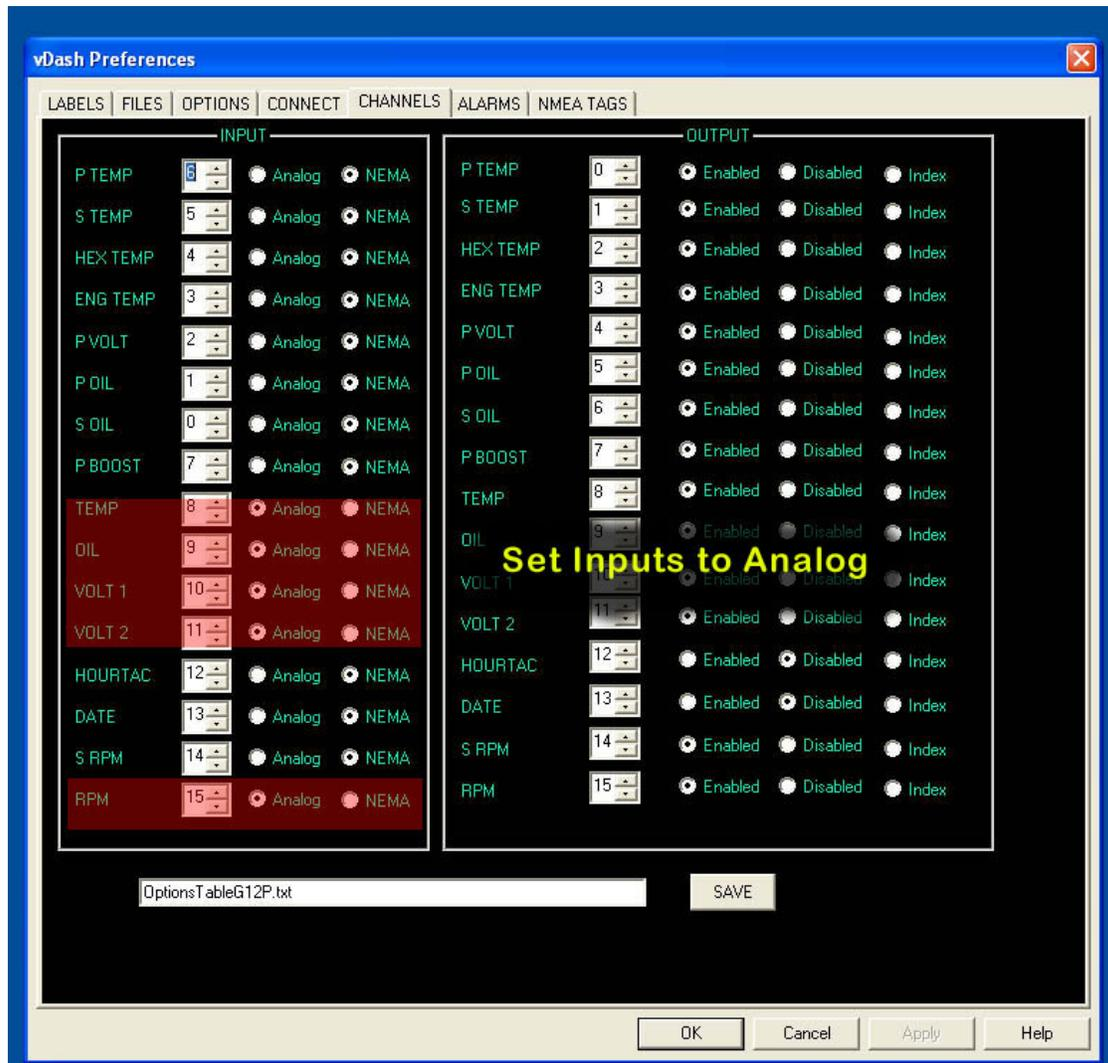
In addition to channel assignment, then Options File is also modified to indicate the number of analog inputs (0-4).
