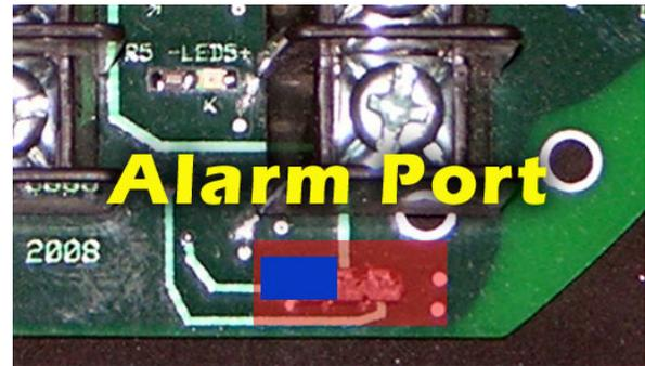
Open Collector Ground drive. Open circuit when alarm off, sink to ground when alarm on. Used to ground relay to drive higher current device. Sinks up to 100 mA
